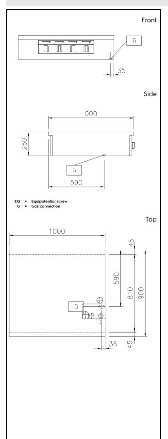
Gas Gas Power: 40 kW Gas Type Option: Gas Inlet: 1/2" **Key Information:** External dimensions, Width: 1000 mm 900 mm External dimensions, Depth: External dimensions, Height: 250 mm Net weight: 82 kg Configuration: One-Side Operated;Top ISO 9001; ISO 14001 - ISO 9001; ISO 14001 kW Front Burners Power: **Back Burners Power:** 10 - 10 kW **Back Burners Dimension -**Ø 70 Ø 70 Front Burners Dimension -Ø 70 Ø 70
